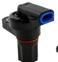
Anti-Lock Brake Wheel Speed Sensors, or ABS Wheel Speed Sensors, play a critical role in a vehicle's anti-lock braking system, as they read and report the speed of a wheel and tire to the ABS Control Module. The ABS Control Module deciphers the data from the ABS Wheel Speed Sensors and uses it for multiple systems like anti-lock braking, traction and stability control and more.
